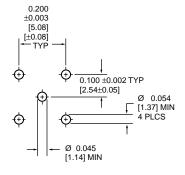
The PCB "footprint" for the 250 Series jack is the same as typically for SMB products. Dimensions shown are "as plated".
